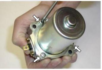
REMOVE DRUM FROM STARTER KEEPING ROTOR IN ITS SEAT (BE SURE TO HOLD THE ROTOR ON ITS TOOTHED SIDE TO PREVENT BRUSHES FALLING OUT FROM THEIR SEAT).
