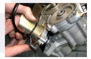
CONNECT THE INPUT WIRING TO THE STARTER WITH THE SCREW M4
