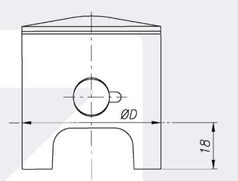
The measure marked on the head of the piston is the real rating.
