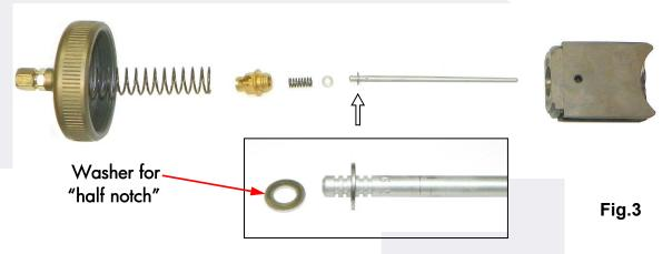
A richer carburetion is got by lifting the needle, by moving down the retainer clip to a lower notch; obviously a leaner carburation is got by lowering it, so moving the retainer clip to an upper notch. (see fig. 3). The basic needle adjustment is shown on the picture.
