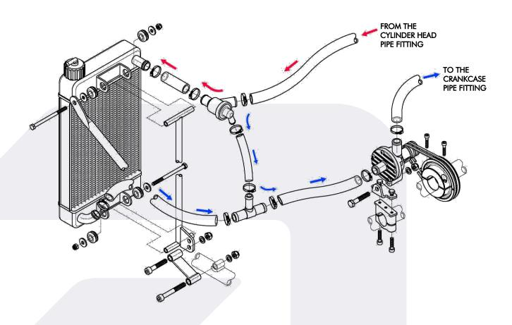
Once the system is filled (with pure water), provide to the good air venting by unscrewing the screw of venting on the cylinder head.
